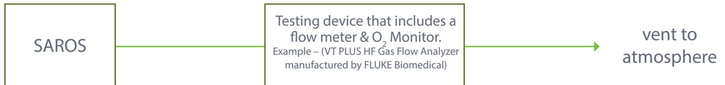
NOTE: If testing concentration or flow rate at multiple settings, allow a 5 minute stabilization period between changing the flow rate prior to taking any test readings.
